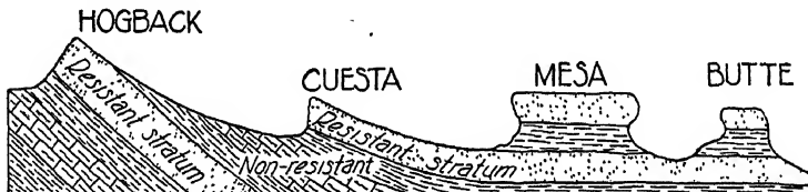
FIG. 124.—Diagram showing the outlines of various physiographic forms produced by differential erosion of tilted and of horizontal beds.
